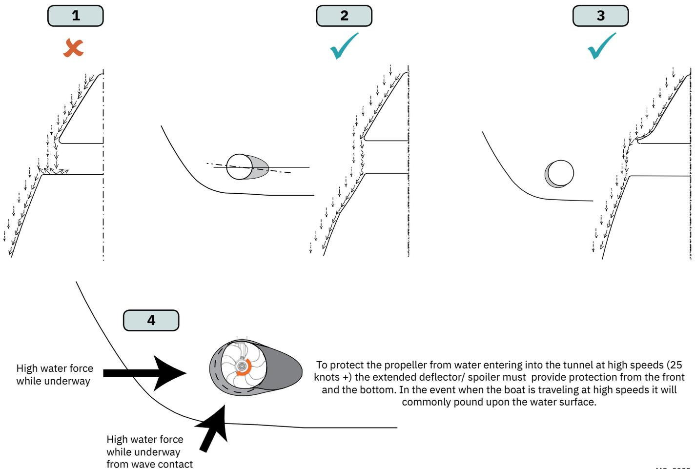
**Rounded tunnel ends will maximise thrust and minimise noise and cavitation.**
