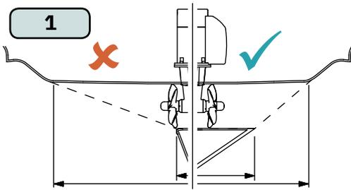
Do not allow the variable length of the tunnel walls to vary in length excessively.
