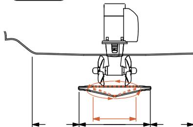
Increase tunnel length to prevent a circular water vacuum cavity between the propeller and the hull of the boat.
