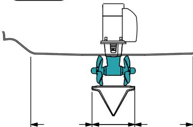
The gear leg/ propeller(s) must never extend out of the tunnel
