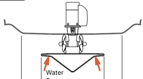
Increase tunnel length to protect the propeller from water forces when high-speed cruising.
