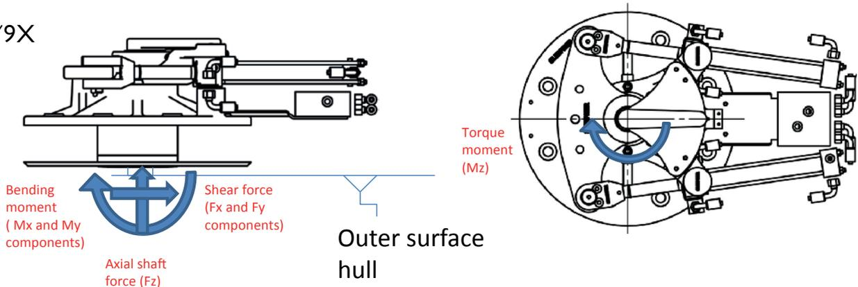
**Note that all calculated values are nominal and found by equilibrium considerations and also that various coefficients are inaccurate as hull design etc will affect the actual fin effect. Dynamic effects such as jumps/impacts with waves, backflow closing of valve etc could further increase the hull/shaft loads. Therefore all dimensioning should account for this by using a safety factor.**
