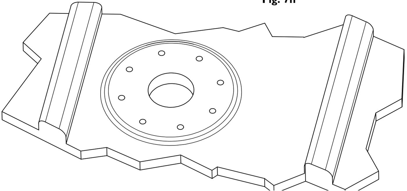
Apply a generous coating of water tight sealant to the mating surface (Fig 7i).
