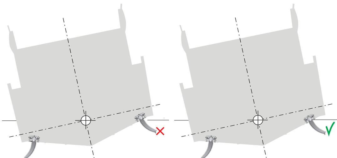
No part of the fin should be above water level during normal roll motion/under normal sea conditions.
