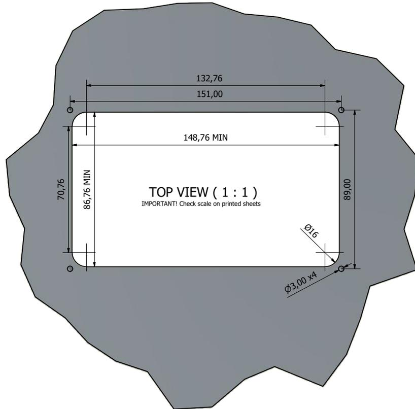
Gasket between dashboard and back surface of panel
