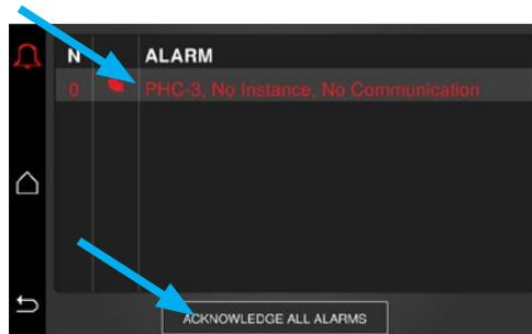
4.3. Touch the active alarm for more details and Correct the cause of the alarm
