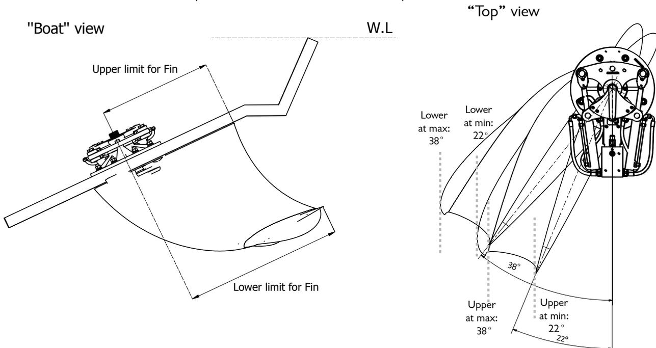
In case of the fin positioning being so that you need to cut down some of the top aft end of the fin to avoid it hitting the hull (very typical on planning boats with hard chines), please do so as per the instructions below.
