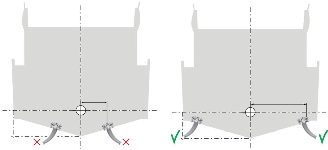
Fins should ideally not extend outside the beam or below the keel when in neutral position.
