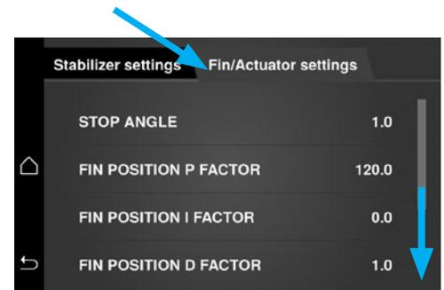
These settings are boat dependant and necessary to achieve optimum performance of the system for a given application. Settings are to be changed only when requested by authorized SP personnel.
