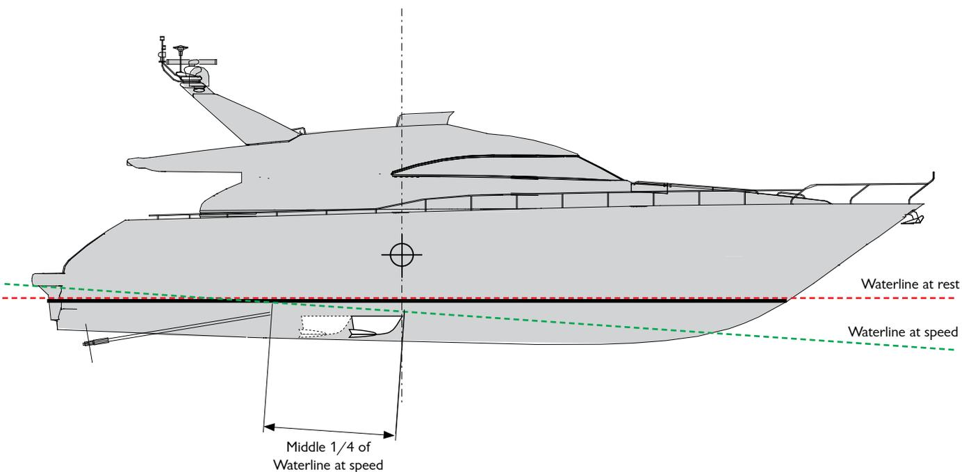
To avoid unwanted influences on the steering characteristics, the fins should be placed close to the vessel longitudinal center of gravity (LCG) - If unknown, this is usually a little aft of 50% of the waterline length.
