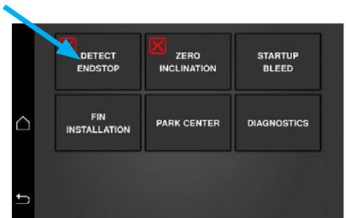
Ensure correct Actuator and Fin type selected.
